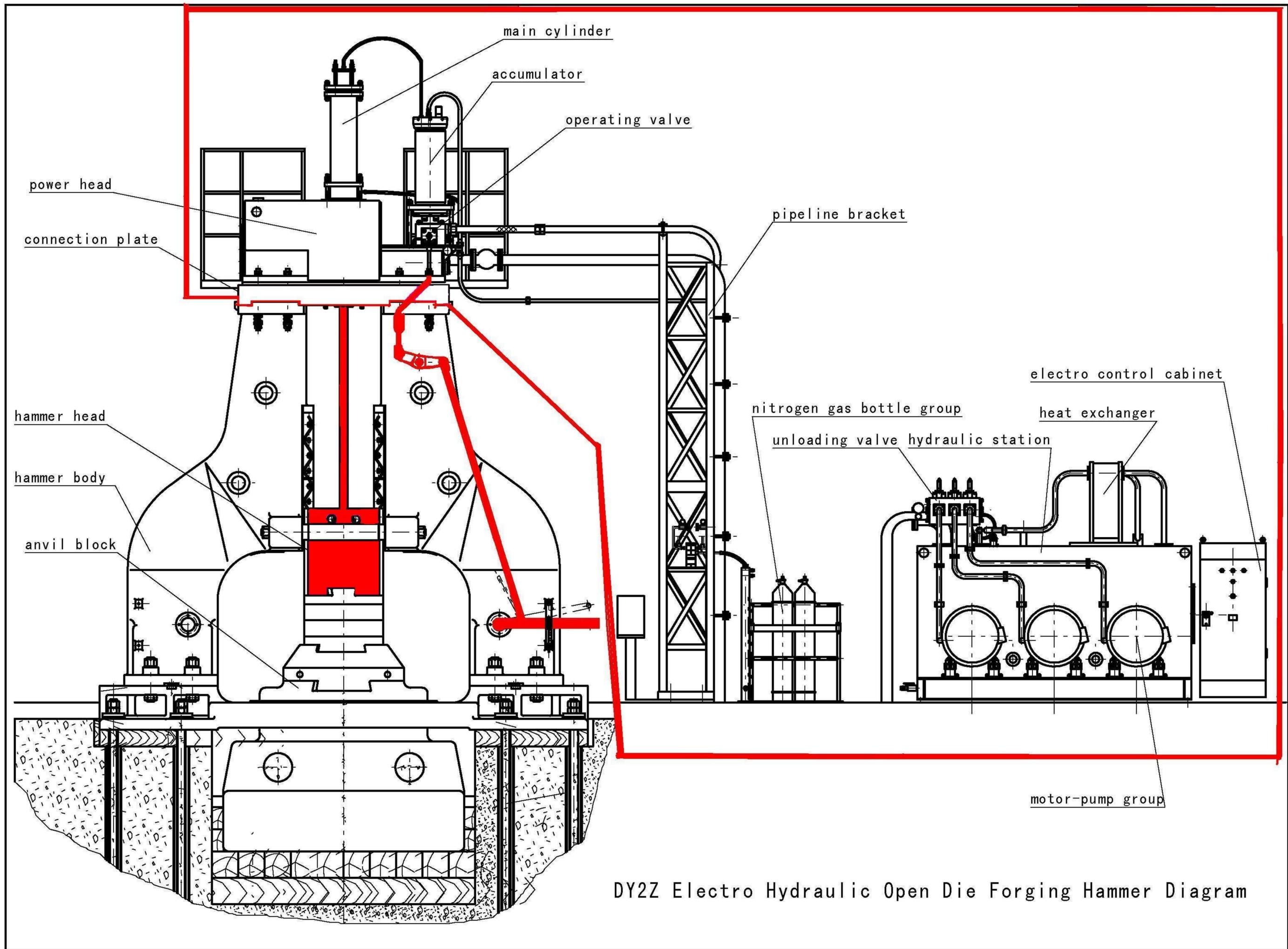
DY2Z Electro Hydraulic Open Die Forging Hammer Diagram
